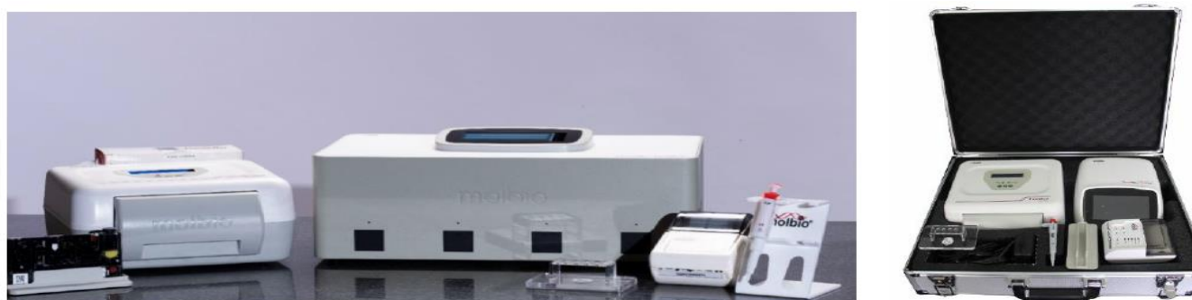
Exhibit 10: Truenat workstation comprising Trueprep/Truelab devices along with accessories
