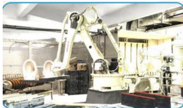
Exhibit 3. Sanitaryware Robotic Glazing
