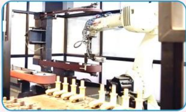
Exhibit 4. Faucet Robotic Surface Grinding
