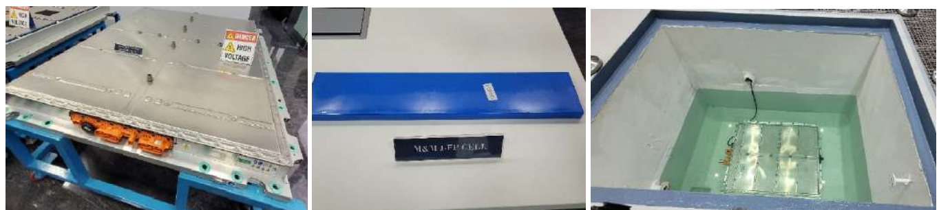
Exhibit 7: Battery cell – BEVs to be equipped with cell to pack advanced LFP blade cell with robust checks
