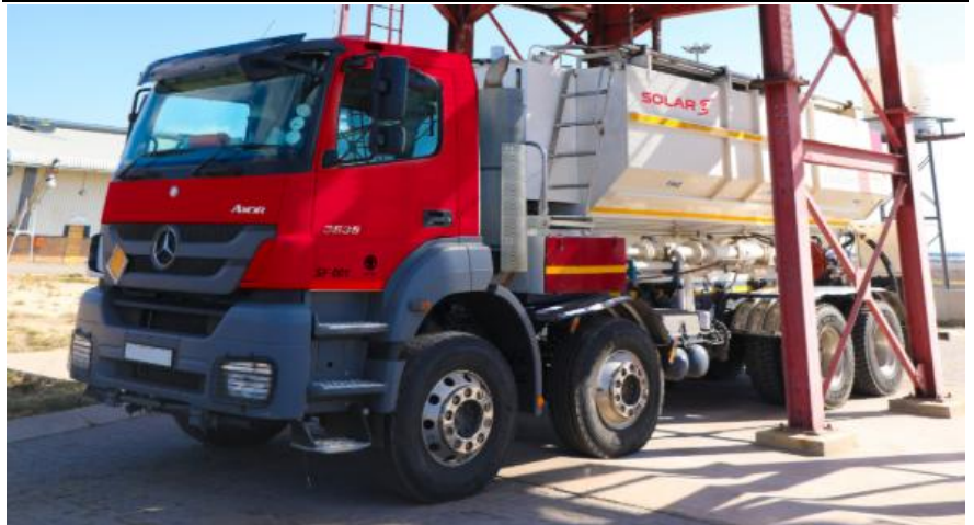
Exhibit 2: Pump truck used to transport bulk explosives
