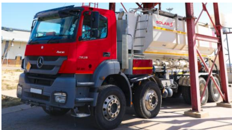
Exhibit 9: Pump truck used to transport bulk explosives
